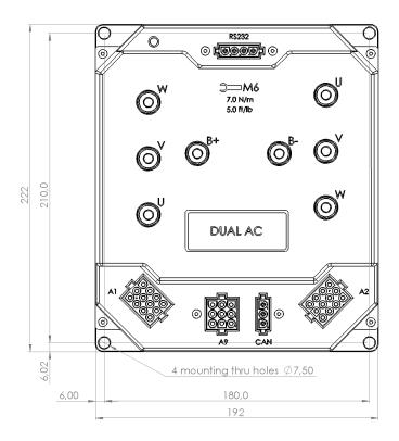
Overall Dimensions 7.6 max" x 8.75max" x2.7" 192 x 222 x 68 mm
