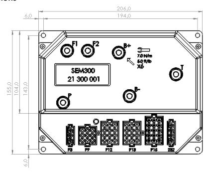
Overall Dimensions 8.12 max" x 6.11 max" x2.7" 206 x 155 x 68 mm
